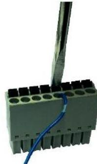
Once the wires are in place, the pair of connector blocks should be connected into the connector adapter on the back of the 8061.
