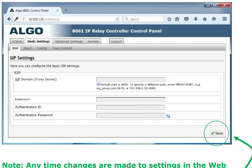
**Note: Any time changes are made to settings in the Web Interface the "Save" key must be clicked to save the changes**
