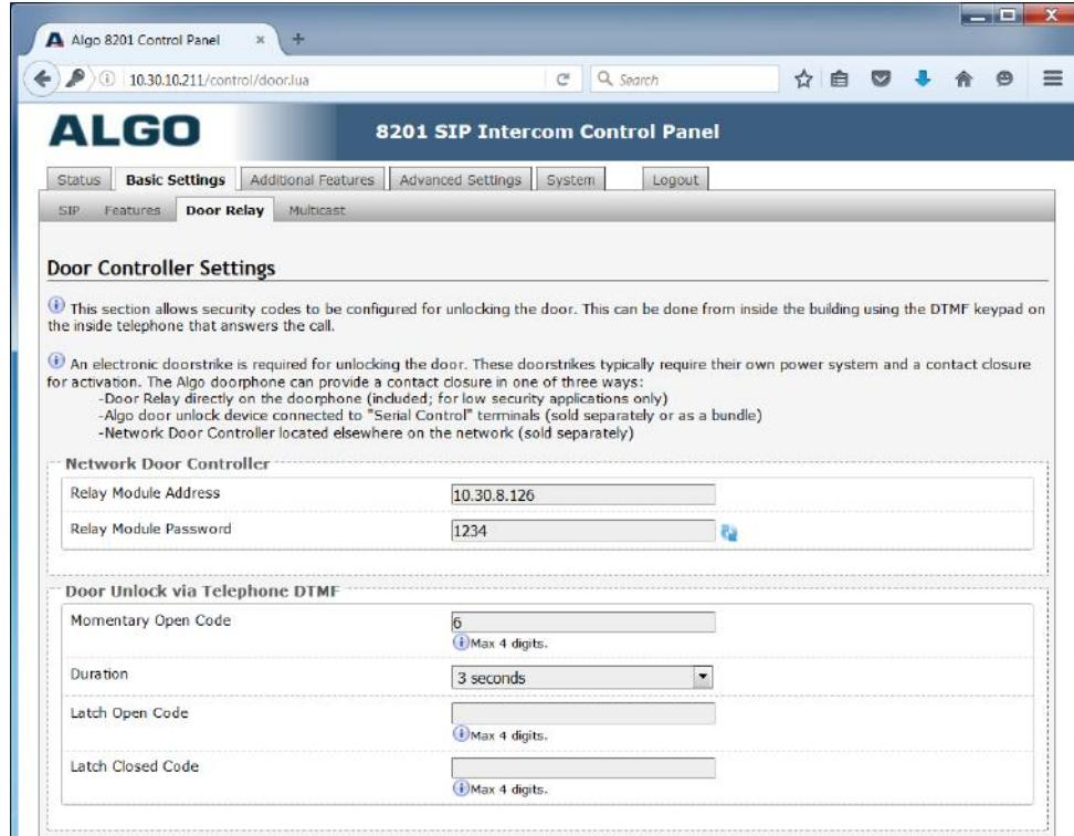
2. Enter the IP address of the 8061 in the "Relay Module Address" field and the associated password in the "Relay Module Password" field. This will be used to authenticate the link between the 8061 and 8201
