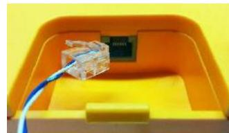
The wire pair can then connect to the **centre pair** of a modular connector at the back of the 1202 Call Button.
