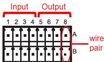
If supported by your phone system, the 8061 can use Subscribe/Notify to monitor up to 2 extensions for events like Ring, In-Use, or both. A specific event on a monitored extension can be configured to one of 4 relay outputs on the back of the 8061.
