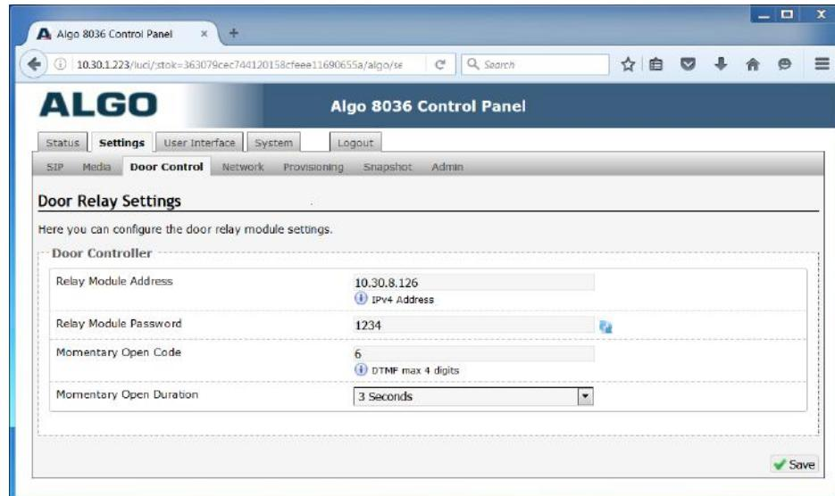
2. Enter the IP address of the 8061 in the "Relay Module Address" field and the associated password in the "Relay Module Password" field. This will authenticate the link between the 8061 and 8036
