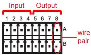
On the adapter, pairs 1-4 are input relays and pairs 5-8 are output relays. Use a screwdriver to depress a push-pin to open the adjacent wire holder (image right).
