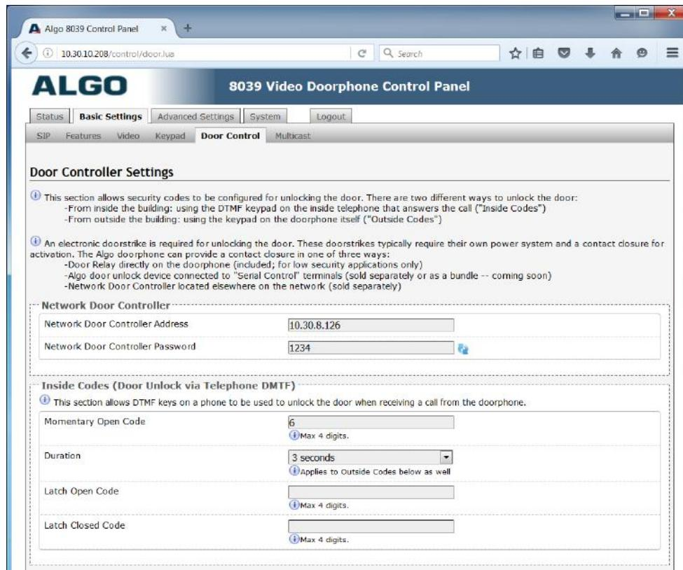
2. Enter the IP address of the 8061 in the "Network Door Controller Address" field and the associated password in the "Network Door Controller Password" field. This will be used to authenticate the link between the 8061 and 8039
