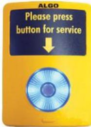
The 1202 Call Button is a one-touch button for event notification and response. It can be used with the 8190S for improved customer service, emergency notification, and non-emergency alerting. The Call Button's one-touch button can trigger a single or continuous action, which can be halted via the small cancel/reset button located below the main call button.
