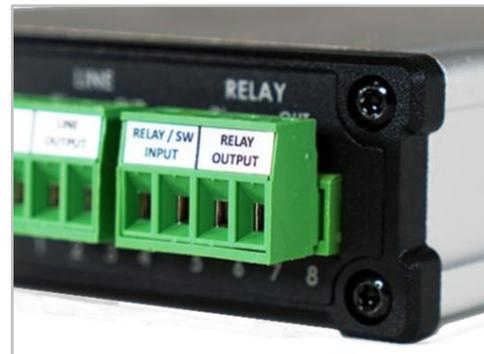
Figure 5: 8301 Relay Input
