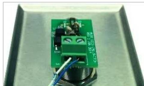
Figure 7: 1203 Call Switch Wiring
