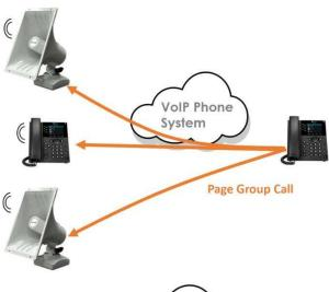
Where the telephone system supports Page Groups and inclusion of a 3rd party SIP endpoint, Algo speakers can be part of this configuration to allow page audio over both telephone and speaker simultaneously.
