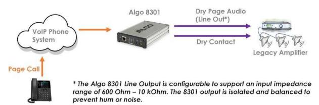
The paging adapters also feature multicast capability to allow for simultaneous audio streaming to Algo IP speakers and to a legacy analog amplifier / speakers as a hybrid paging system.
