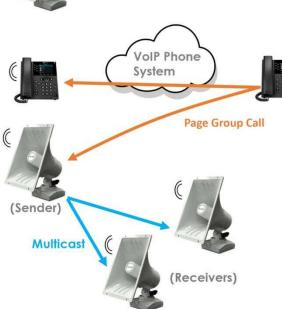
If desired, the Algo speaker can also be configured to multicast to include more endpoints as part the Page Group call. This is particularly helpful where there is a limit to the number of extensions permitted in a Page Group and additional speakers are required to provide coverage over an area.
