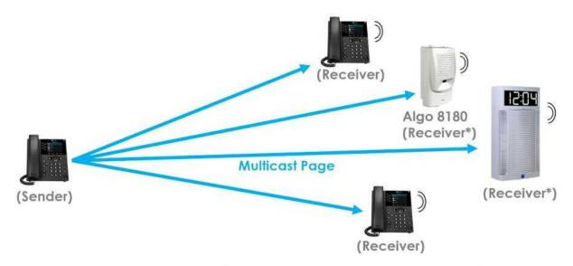
\* No SIP registration required for Receivers in a multicast.
