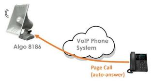
Integrating to a VoIP telephone system or unified communications (UC) platform, the Algo speaker is an endpoint like any other IP telephone. In the simplest configuration, the speaker is activated by calling an extension associated with it on the telephone system. Within the Algo endpoint this is referred to as a *Page extension* which is designed to autoanswer when called. Any device in the UC
