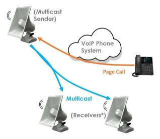
\* No SIP registration required for Receivers in a multicast.
