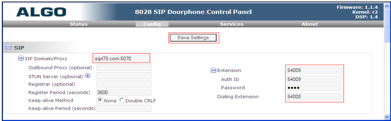
Figure 21: Configuring the SIP Doorphone Control Panel
