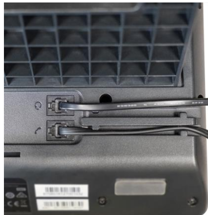
Figure 5: Connection from RJ9 to headset
