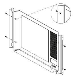
4. Install the polycarbonate sheet using the 10-32 attachment screws and aluminum spacers. Ensure the rectangular cutout is aligned to the speaker grill of the 8410.
